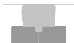
Installation flush with ground
