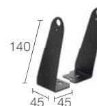
WMA02N Pair of brackets h 140 mm (Neva 3 / 4)
